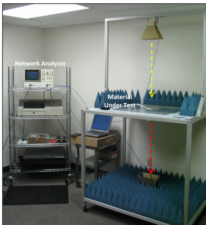
Figure 1. Overview of Transmission Tunnel Test Setup
